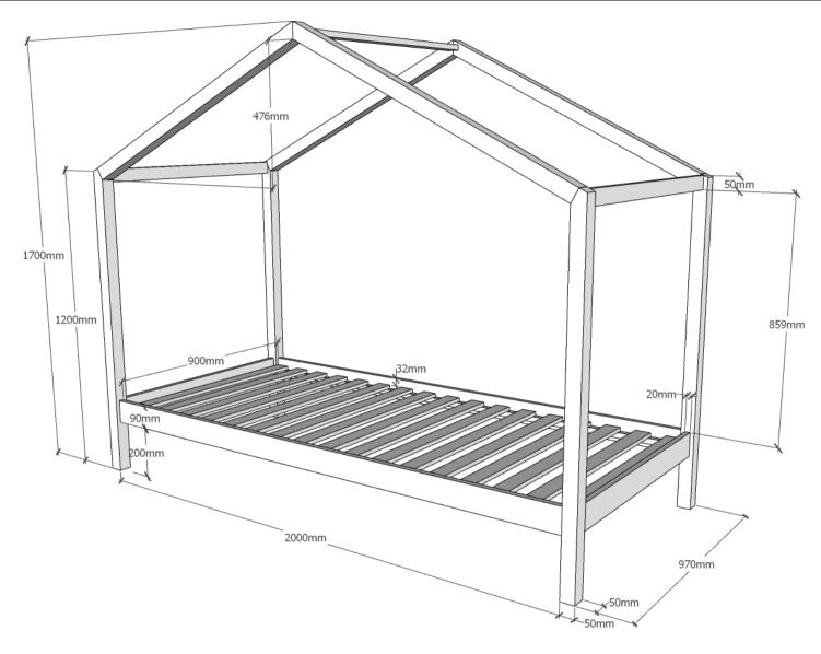
L:2100mm H:1700mm D:970mm innersize 900x2000mm
